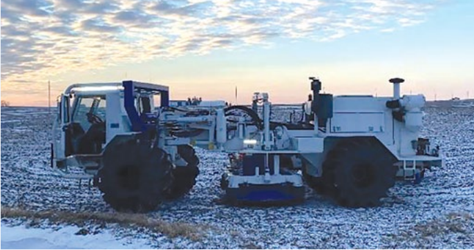
Vibroseis truck in Illinois. Photo Credit: Allan Châtenay, Explor. (Explor CCUS project in Illinois, 2022)
